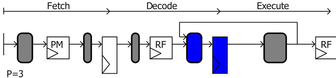
Figure 5.3: Pipeline stages and register file write-through short cut.
