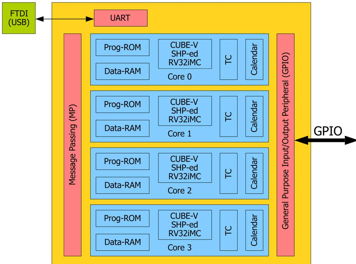
Figure 5.1: Overview of the FPGA design.
