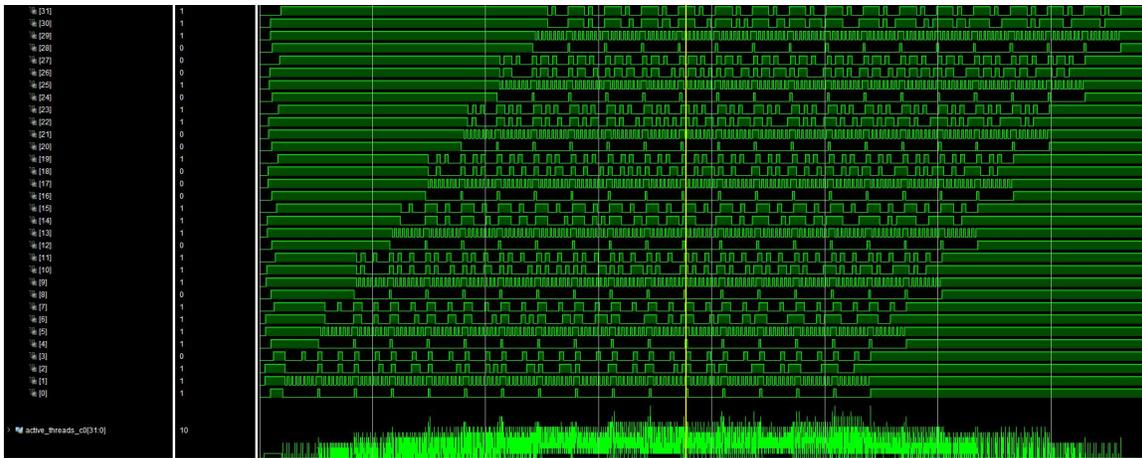
Figure 7.1: Running 8 SPI master and 8 SPI slave virtual peripherals from one core.
