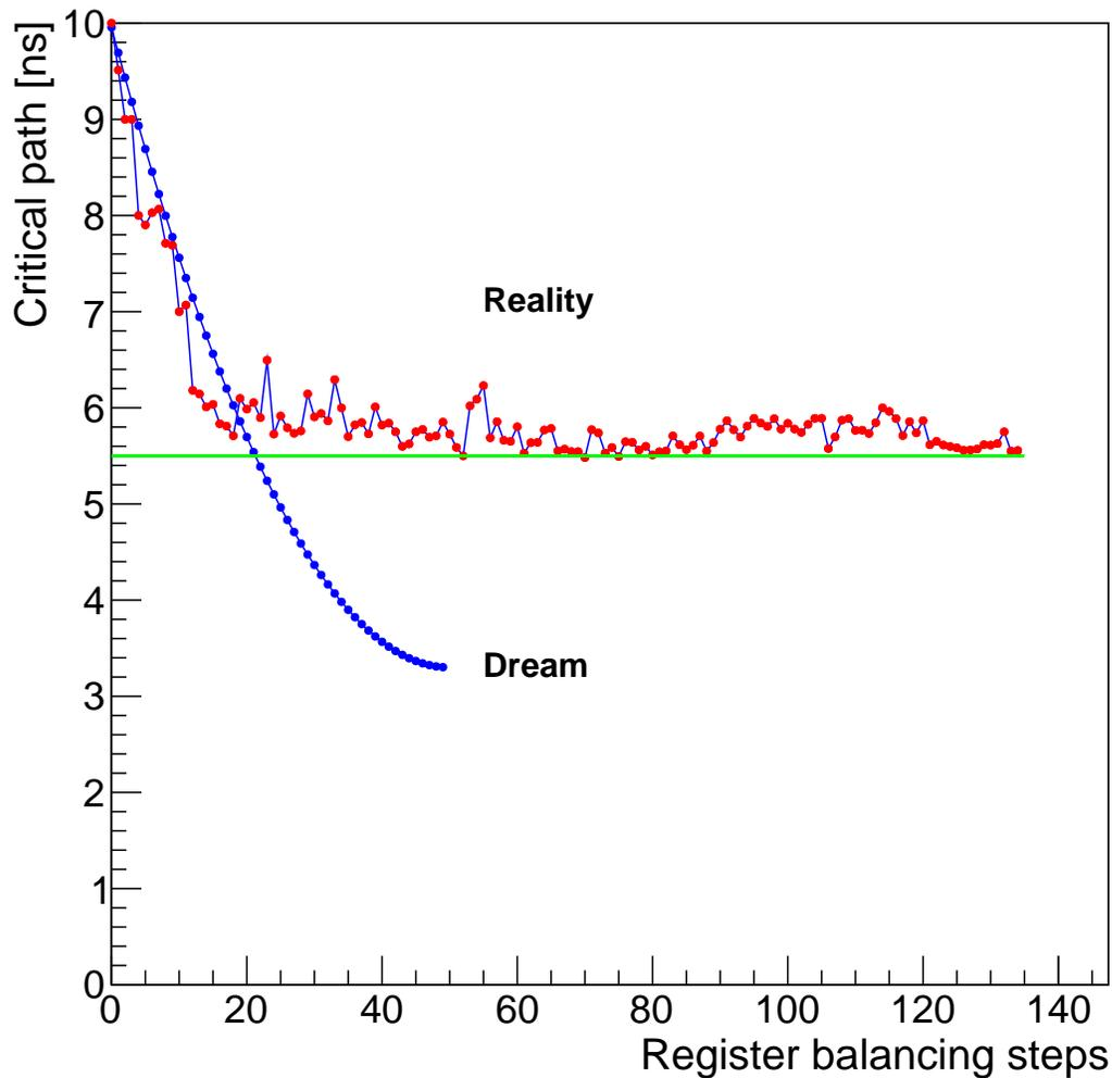
Figure 5.2: Register balancing steps of SHP-ed RV32iMC on Artix-7.
