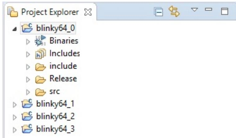
Figure 8.2: Project's postfix indicate individual core.
